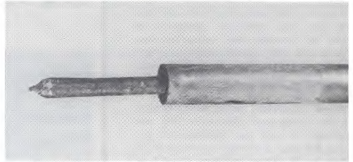
A dirty, badly shaped soldering iron tip can lead to bad solder joints. Reshape and clean tip.
